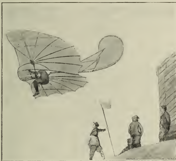
Otto Lilienthal Experimenting with His Flying-Machine: Starting from a Platform.
